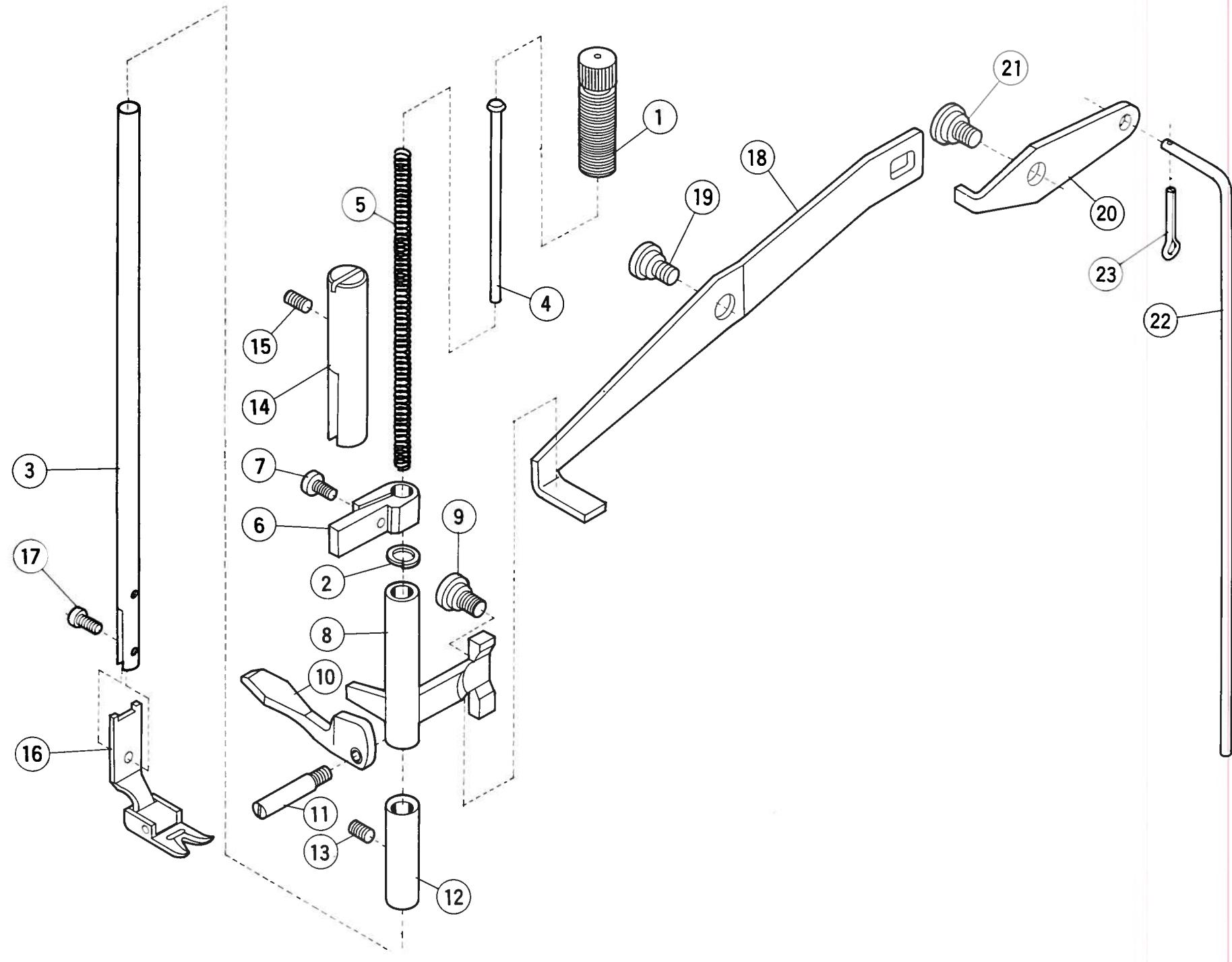
**PRESSER FOOT AND LIFT MECHANISM**
