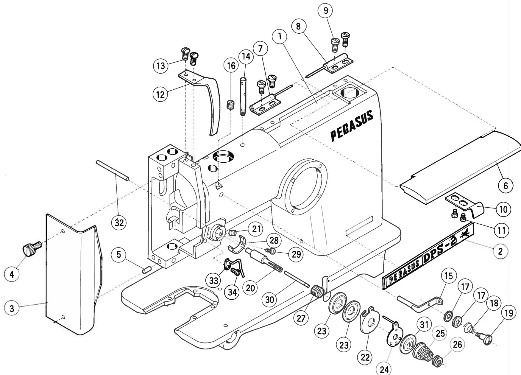
**MACHINE ARM-BED, FRAME COVERS & NEEDLE THREAD PARTS**
